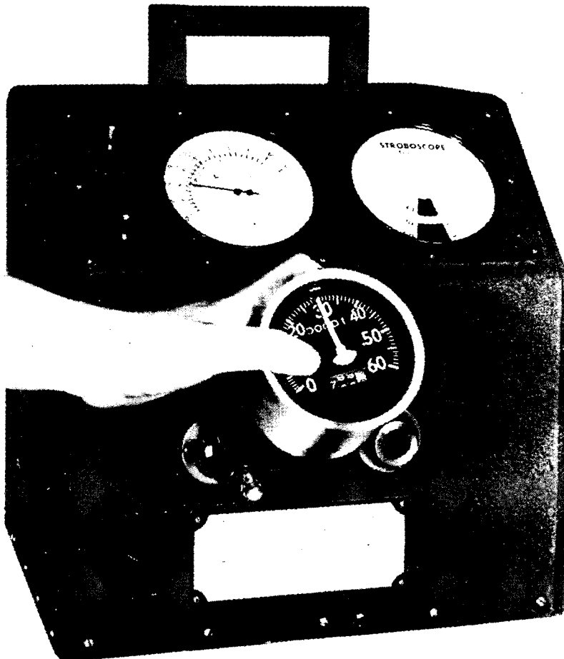
Figure 73—Holding Speedometer on Calibrating Machine (T-170645) and Testing at 30 mph
